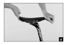
Once you have found the desired position, tighten the two bolts alternately and gradually by using a torque wrench (a) to the maximum torque value indicated in Nm on the AX-Lightness and engage seat post.
