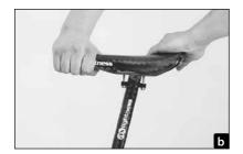
Make sure the lever is fully closed. Only in this position maximum hold is achieved and it is ensured that the quick-release remains closed.
