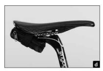
Having found your preferred position, make sure both brackets and the lower holding cup of the clamping mechanism fit snugly around the saddle rails (a) before tightening the bolts to the indicated torque value.
