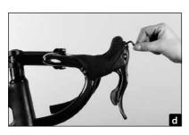
In the case of road racing bicycle brake lever/shifter units (Dual Control, Ergopower or DoubleTap) dismount the clamp completely from the unit (a).
